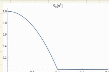
Figure I: Litim propagator  $R_K(p^2)$
