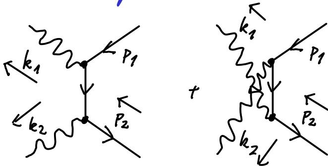
The amplitude for this process can be obtained from the one for Compton scattering by making the replacements  $p \mapsto p_1$ ,  $k' \mapsto k_1$ ,  $p' \mapsto -p_2$ ,  $k \mapsto -k_2$
