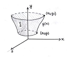
Consider two points on the xy-plane  $(x_1, y_1)$  and  $(x_2, y_2)$  connected by a cartesian curve y(x). Find the function y(x) that minimizes the surface  $J\{y(x)\}$  obtained by rotating the latter around the y-axis.
