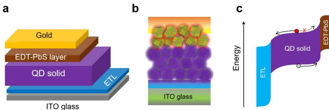
**Figure 2.** a) Classic planner structured QD photovoltaics device architecture and b) the cross-sectional QD stacked sketch, in which a QD solid acts as the active layer in a sandwich structure between the hole transport layer (which is normally a thiol treated QD layer) and electron transport layer. c) Energy diagram indicates the working principle of the PV device.
