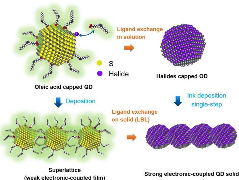
**Figure 1.** Schematic of the ligand exchange of QDs in solution and in a solid-state QD film, in which the ligand exchange converted the QD film from a weakly electronically-coupled superlattice into a strongly electronically-coupled mode.
