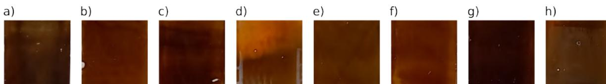
Figure 8.4: Photographs of the  $\text{MAPbI}_3$  films with the solvent system a) DMF/DMSO, b) GBL/DMSO without additive, c) GBL/DMSO with MAI as additive, d) GBL/DMSO with MABr as additive, e) GBL/DMSO with tBP as additive, f)-h) GBL/DMSO with MACl (low, medium, high concentration) as additive.
