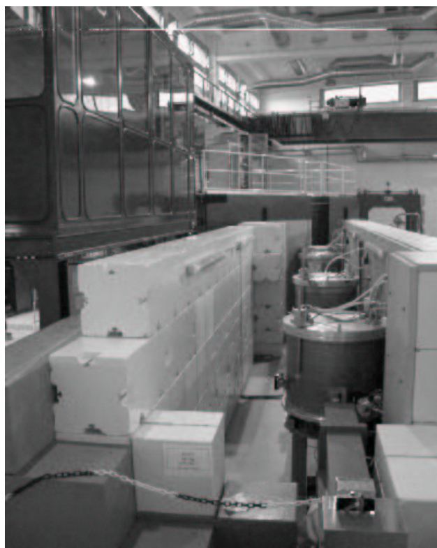
Abbildung 1.1: Front view of the time-of-flight spectrometer at FRM-II with disassembled shielding of the primary spectrometer (see text)
