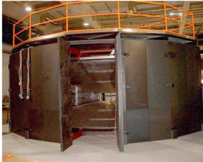
Figure 1.4: Flight chamber of the TOFTOF spectrometer
