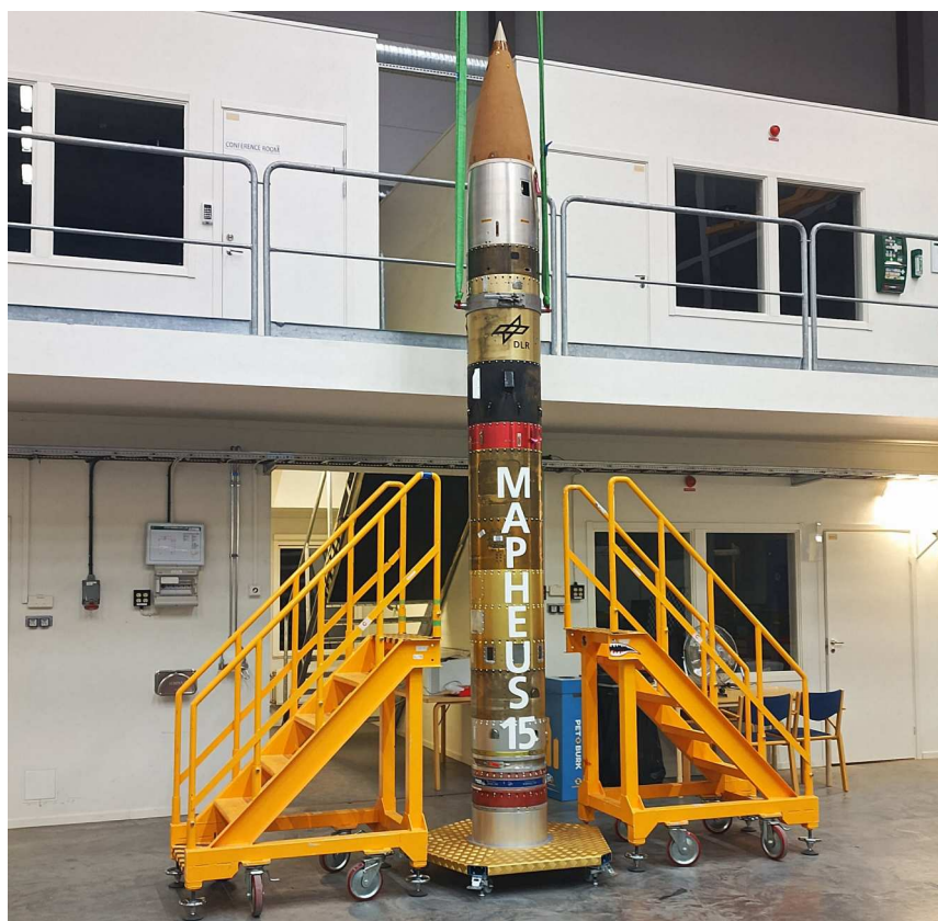
Figure 8.3: Photo of the fully integrated payload. The SVAL*IN experiment is located towards the bottom of the payload at the height of the letter "U".
