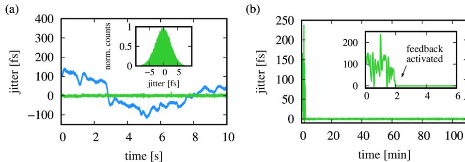
Fig. 2. (a) Short-term timing jitter unsynchronized (blue) and with active synchronization (green). The RMS timing jitter in the stabilized case is reduced to  $\sigma < 3$  fs. The inset shows a histogram of the measured timing jitter values. (b) Long-term measurement of the timing delay between the pump and seed pulses. Inset: Activation of the stabilization after 2 min.
