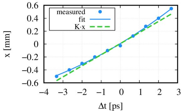
Fig. 1. System calibration curve. A second order polynomial fit is applied to the measurement. The tangential slope at  $x = 0$  mm yields the calibration factor  $K$ .
