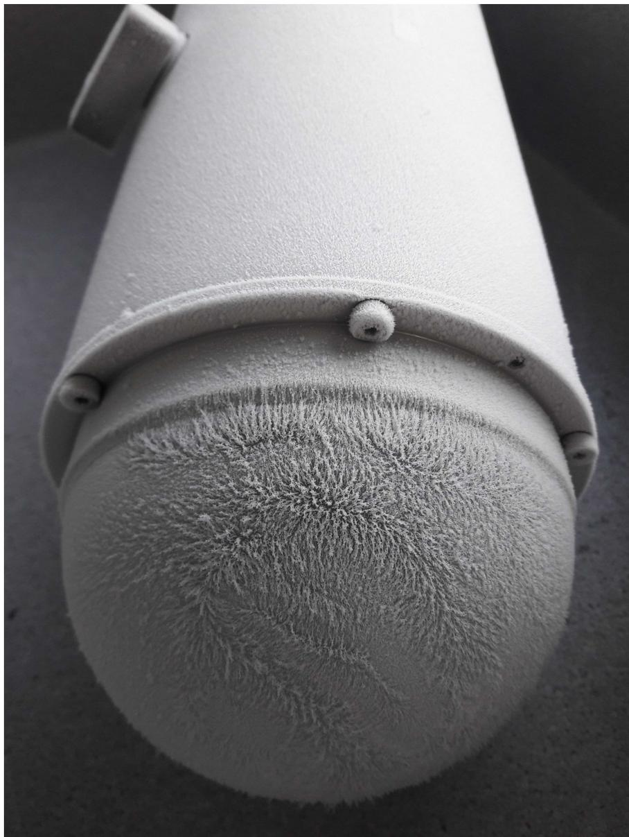
Fig. A.1: Picture of the POCAM after cooling it down to  $-80^{\circ}\text{C}$ . The formation of ice crystals on the surface started immediately after exposing it to room temperature.
