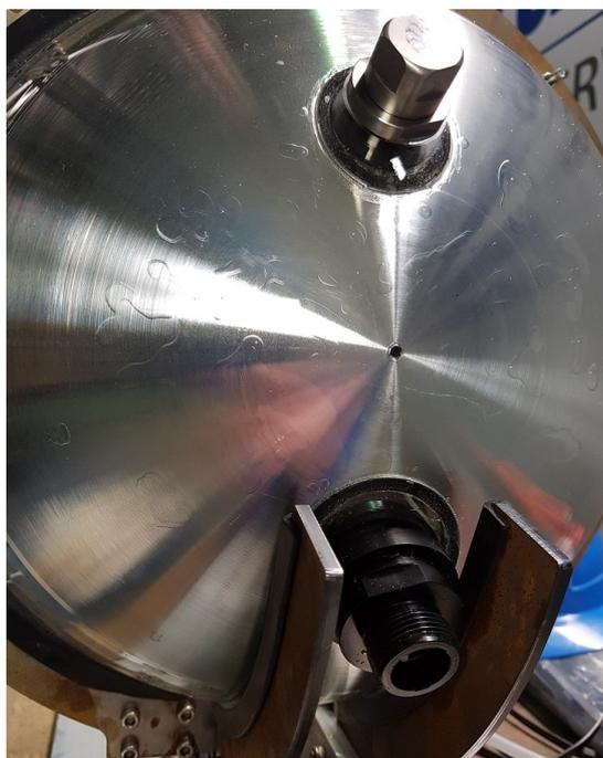
Fig. A.16: Pictures of the standard module assembly after the pressure test. The lower picture shows the gel detachments.
