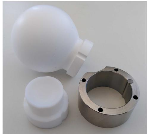
Fig. 3.2: Picture of the PTFE-sphere and the aperture disk mounting ring. To account for different thermal expansion coefficients the mounting ring is designed smaller and the sphere is fitted in after cooling it down to  $-50^{\circ}\text{C}$ .
