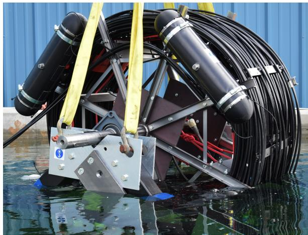
Fig. 4.1: Photography of a mooring line assembly hosted on the winch, as it was lowered into the test pool of ONC. Picture taken by Felix Henningsen.
