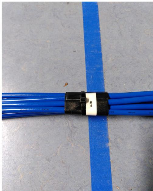
Fig. A.8: The hybrid cables foreseen for the deployment of STRAW-b have been bundled again and wound up on the instrument tray. This was performed in a hallway of the physics department, where the floor was marked every 12 m. At these markings, the bungee cords and respective position marks were attached. Upper picture taken by Elisa Resconi.
