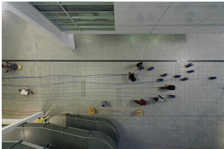
Fig. A.7: The VEOC was delivered in a bunch of fourteen cables. For testing and handling, the individual hybrid cables were separated on single spools. This operation was performed in the main corridor of the engineering department, where the cables could be stretched out over a large distance to handle their internal strain and twists. Pictures taken by Kilian Holzapfel.
