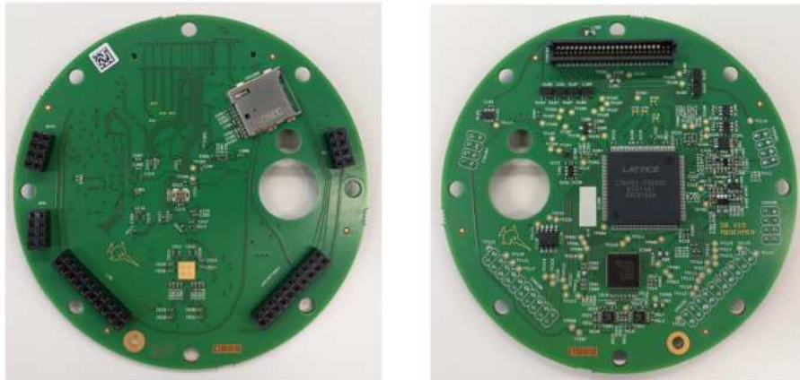
Figure 4.5.: Top (left) and bottom (right) view of the digital board (DB).
