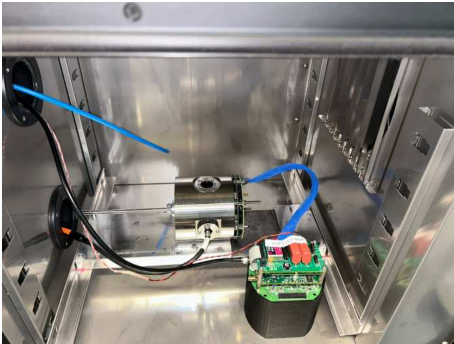
Figure 5.7.: Characterization stage inside the freezer with an exemplary set of the necessary components that had to be installed.
