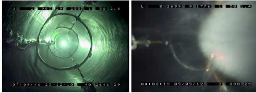
Figure 3.6.: Photos of a drill hole for a string deployment right before refreezing (left) and how the cloudy hole ice (right) looks like after has frozen again.
