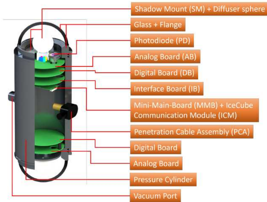
Figure 4.2.: The figure is a schematic cross-section of the POCAM showing its internal (electrical) structure. Figure taken from [10].
