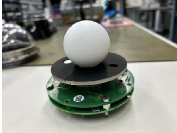
Figure 5.6.: Hemisphere stack to be mounted into the characterization stage inside the freezer. It mainly consists of a diffusing sphere, a shadow mount as well as an analog and digital board.
