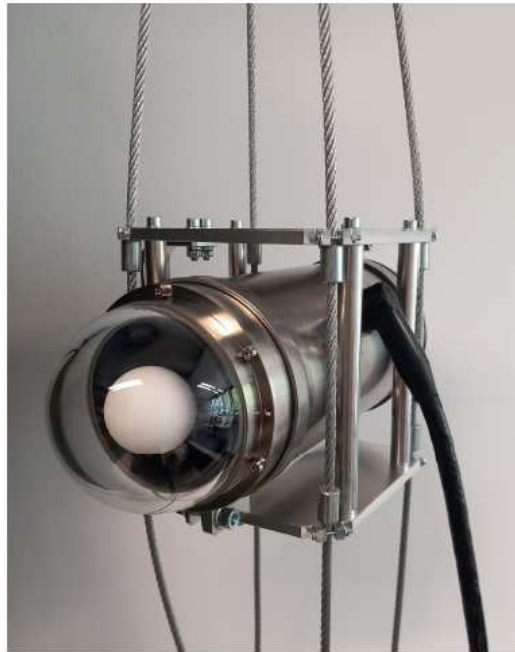
Figure 4.1.: Fully assembled POCAM device mounted into the harness by which it will be attached to the deployment strings via steel ropes. Beneath the glass hemisphere the diffusing sphere can be seen which is mounted onto a coated surface and is responsible for an isotropic light emission.
