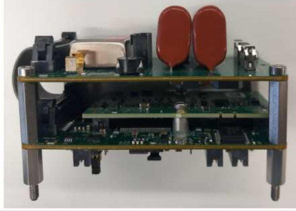
Figure 4.3.: Mini-main board (MMB) stack, with the board dealing with power conversion on top, the control board at the bottom and the ICM connecting both in the middle.
