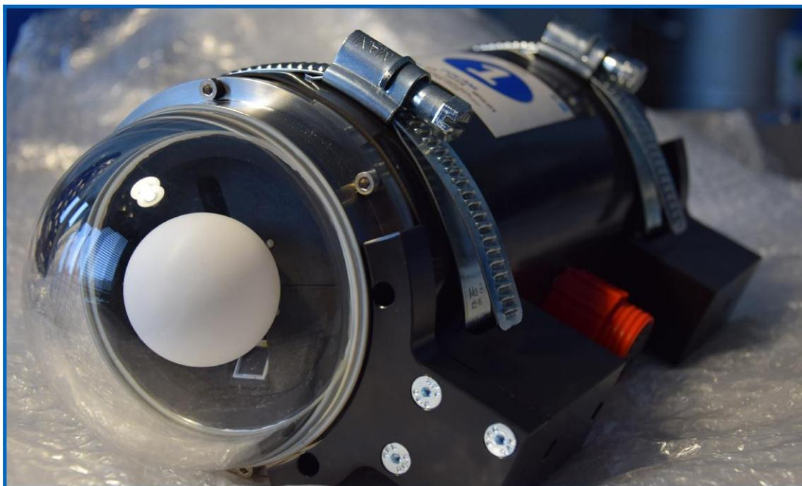
**Figure 4.26:** Finished POCAM module for STRAW. In addition to the instrument itself the mounting structure for the holding structure is visible.
