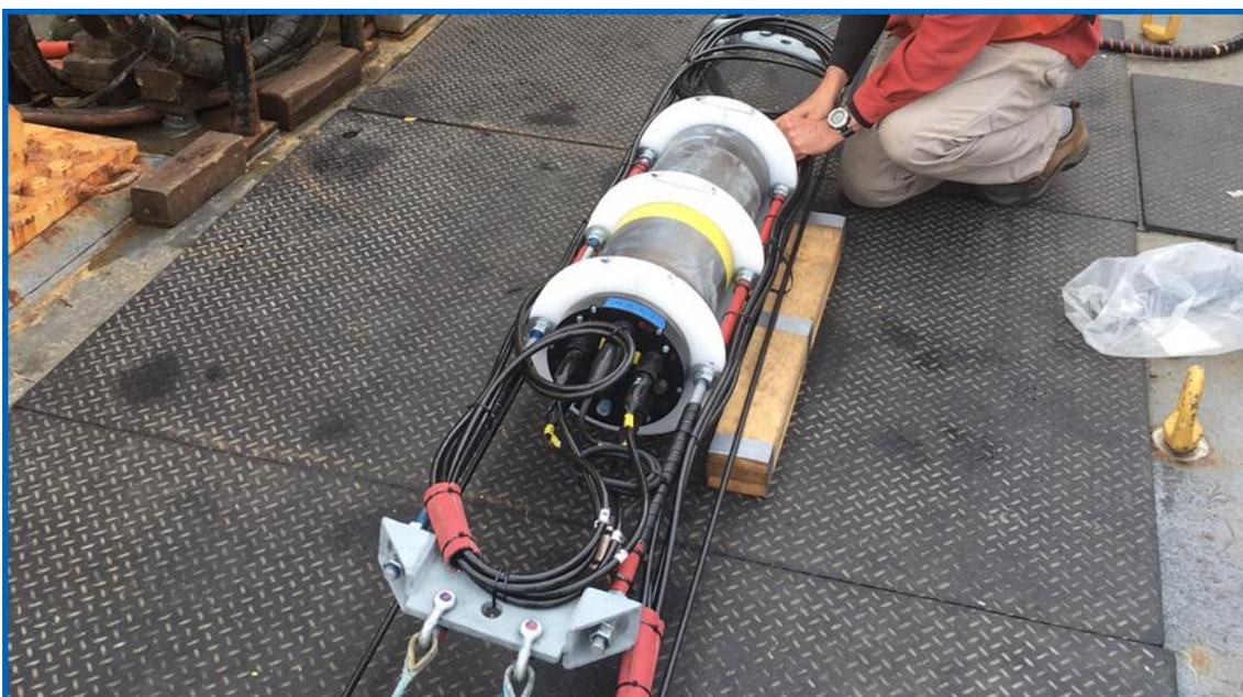
Figure C.3: On-ship mJB mounting to a STRAW string. Courtesy of P. Macoun, ONC.
