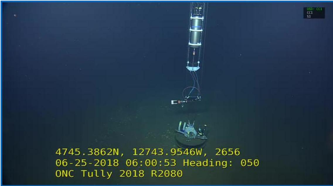
Figure C.6: ROV inspection: mini junction box. Depth: 2656m.
