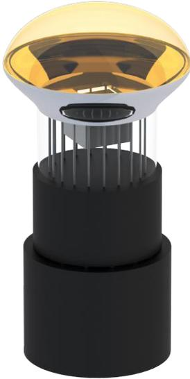
The detection principle of a photomultiplier relies on the photoelectric effect, that is, the emission of electrons upon incident light on the photocathode. Using an applied high voltage (HV), such *photoelectrons* (PEs) are then accelerated through the dynode chain and multiplied at each stage by collision-ionization. This way, an incident electron can be amplified by  $10^5 - 10^8$  in charge until arriving at the anode where the signal is measured.
