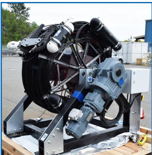
**Figure 6.2:** Spooling system of a STRAW string. The instruments and the engine are visible.
