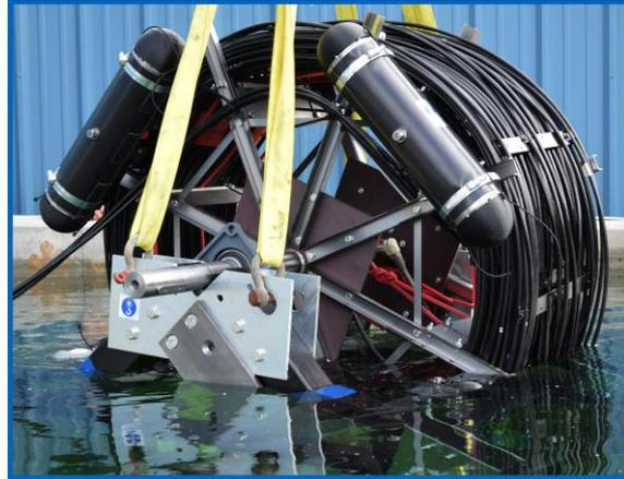
**Figure 6.3:** STRAW assembly being submerged in the ONC test tank using a heavy lift crane.
