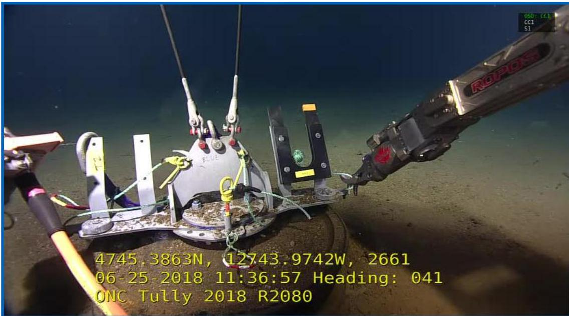
Figure C.7: ROV rotating anchor. Depth: 2661m.
