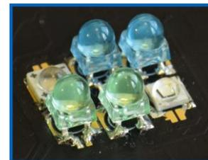
**Figure 4.4:** POCAM prototype LED layout.
