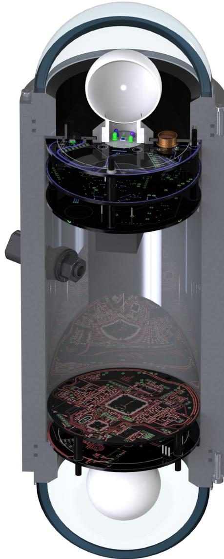
Figure 3.6: Cutaway drawing of the full POCAM for GVD. Both hemispheres have a set of one analog (with the mounted integrating sphere), and digital PCBs and the fifths provides the power supply. Each side has 6 LEDs (upper center), a SiPM (left of LEDs), a Pin-Diode (right of LEDs) and amplifiers. The digital part provides, the trigger and DAQ as well as the communication with a  $\mu$ -controller and FPGA.
