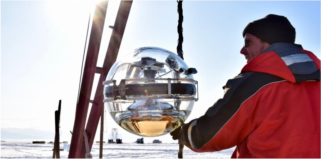
Figure 2.4: *The Optical Module in GVD has a 10-inch PMT (golden), which is mounted inside a 17-inch pressure-resistant glass sphere. Between the glass sphere and the PMT an optical gel avoids total internal reflection. Therefore, the PMT appears so big on the photo. All electronic components inside the OM are attached to the base of the PMT. In subsection 2.2.1, the OM is explained in more detail. This photo was taken by F. Henningsen during the deployment in March 2017.*
