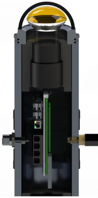
Figure 4: This is a cross section of an sDOM. The sDOM contains 2 PMTs, one at each end. The electronics are capable of handling both at the same time. The 3D render was kindly provided by Felix Henningsen.
