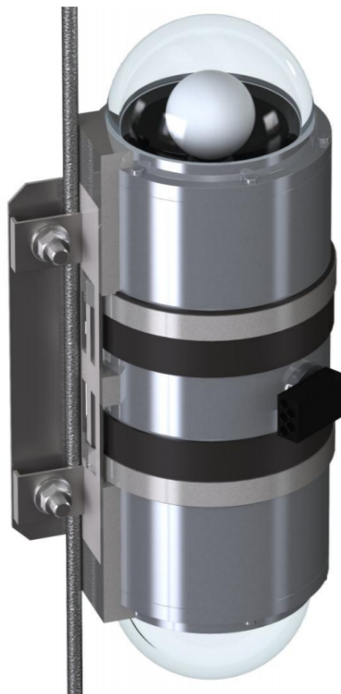
Figure 3: This is a 3D model of a POCAM. The POCAM contains 2 LED arrays, one at each end. The 3D render was kindly provided by Kilian Holzapfel.
