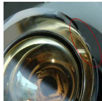
Figure 2.17: Here the gel flowed out strangely and creates this folded structure at the edge of the gel pad but couples fully nonetheless.
