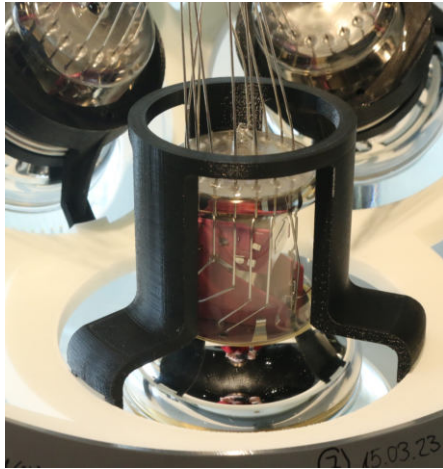
Figure 2.7: The alignment tool holds the PMT in place without putting pressure on it. This makes sure the PMT and gel pad are perfectly aligned in the hemisphere.
