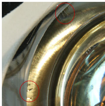
Figure 2.16: When using too much gel sometimes tree structures form on the surface of the gel pad.
