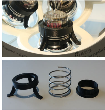
Figure 2.8: The holding structure holds the PMT in place and is applied after the gel is cured. It consists of a lock that is seized into the white frame, a spring, and a collar, all placed around the neck of the PMT.
