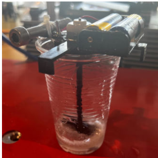
Figure A.4: View from the outside of the vacuum chamber. The automatic stirring device mixes the gel while degassing.
