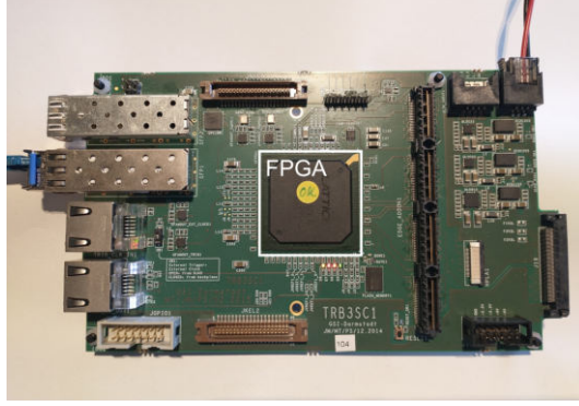
Figure 3.2: The used TRB3sc board with the FPGA right at the center. The signal out and input are on the left side where the fiber is connected to the board. The red and black cable provides power to the board.
