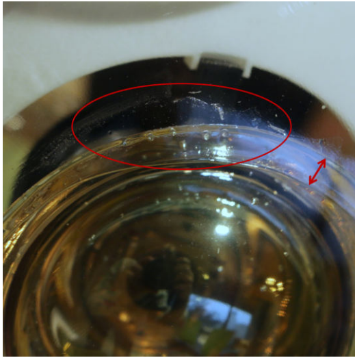
Figure 2.11: The interface gel in this integration at first flowed out enough but came back during the curing process, leaving the edges of the gel pad with not enough gel for a complete coupling.
