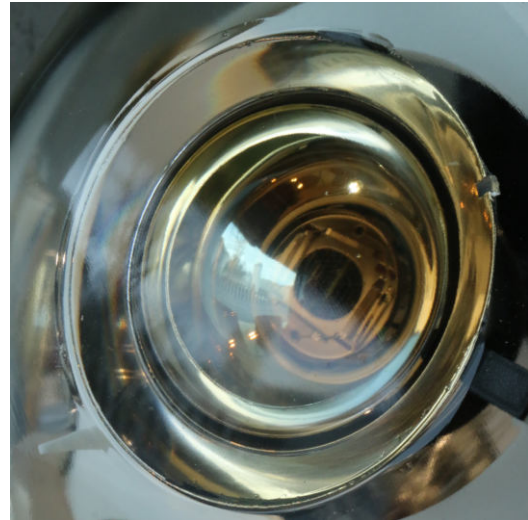
Figure 2.14: This gel pad is coupled fully to the hemisphere with only a little amount of interface gel flowing out on the sides. However, the overflow is not even: on the top right edge of the gel pad no overflowing gel is visible.
