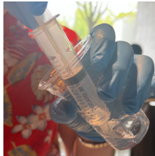
Figure A.5: The syringe is drawn up to more than 7 g. With a small amount of gel this must be done carefully to not produce bubbles in the process.
